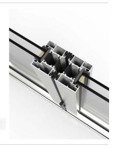
Thermally broken system with 73 mm of frame depth, ideal to divide environments and unify spaces both in residential and commercial buildings. It allows multiple combinations of up to 14 sashes that allow to close spans of more than 16 meters wide. It has slim sightlines and hidden rollers, showing a clean aesthetic in the closed position. In addition, the flush threshold facilitates accessibility and transit between the interior and exterior.
